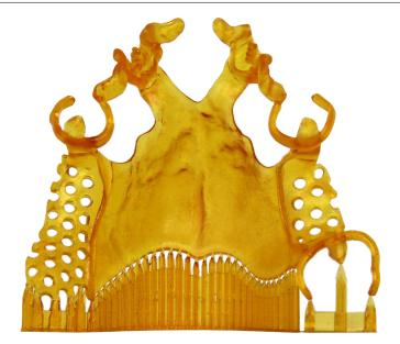
EnvisionTEC's E-Partial chemistry was developed for building partials where some flex is required. E-Partial material maintains flexural strength to ensure clasp flex without breakage. The stiffness of the material allows for the production of a very hard retention grid and super tight thin clasps to deliver a metal partial with the perfect every time.
